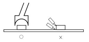
■ Avoid rubbing or scraping the resin by any object, during high temperature, for example reflow
