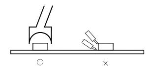
■ Avoid rubbing or scraping the resin by any object, during high temperature, for example reflow \ solder etc.
