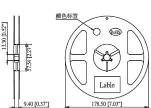
Dimensions of Tape (Unit: mm)
