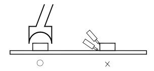
■ Avoid rubbing or scraping the resin by any object, during high temperature, for example reflow \ solder etc.
